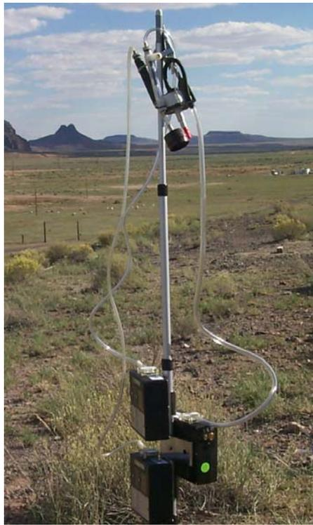
**Figure A5. Assembled samplers for dusts and SVOCs**
